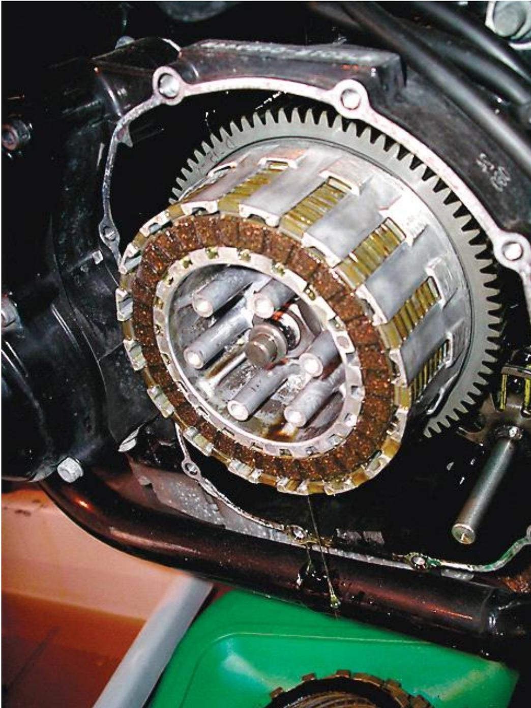
10 Refit the pressure plate - it may only go on in one position - and fit the new springs. Do up the bolts to the specified torque setting
