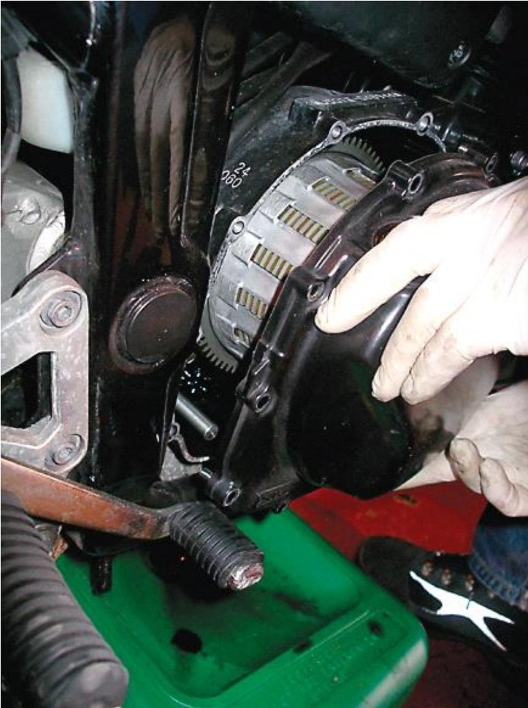
3 The old gasket should come off in one piece. If not, use a gasket scraping tool. Don't hack away with a screwdriver or you might damage the casing and it won't be oil tight
