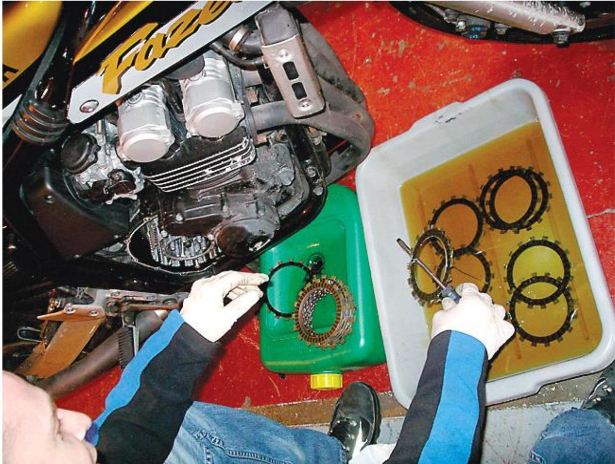
9 ... and repeat until it looks like this. Ensure you put in as many friction plates as came out, but don't worry if there are new friction plates left over - some kits provide more than needed
