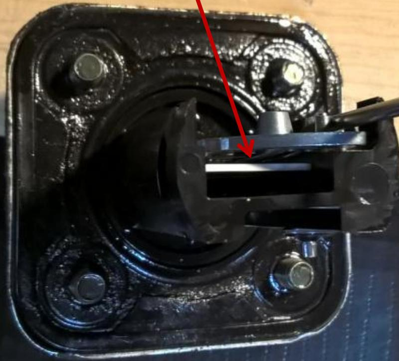
Open ended spanner under bar via slot
