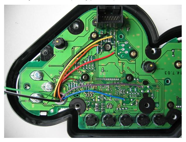
14.) Pull double black cable (ambient temperature sensor) and the optional green control cable through the hole in the cluster's rear wall before reassembling the cluster. Check the correct alignment of the gauge relative to the other instruments. Close the housing with 7 srews.
