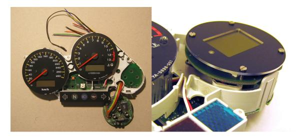
To protect the needles and surfaces use the upper part of the housing to carry the instrument from now on.
