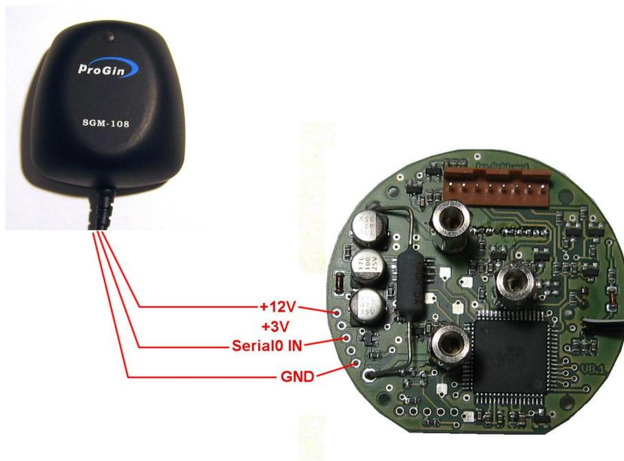
The NMEA signal goes to serial input #0 of the processor only. *Serial0 OUT* is not used as the multi gauge is a listen-only device.
