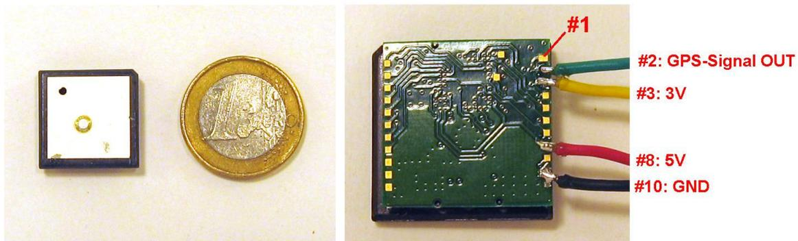
This module is very tiny. It needs an additional low current 3V supply at #3 as reference for the I/O signal level (the Multi Gauge is capable to deliver this).
