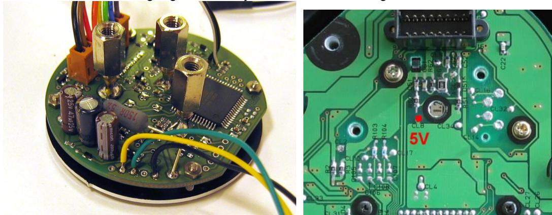
The most simple way to get a 5V supply is to tap the existing cockpit supply at "CL8" (or somewhere on the copper plane nearby). This supply is strong enough to also support an additional GPS module.
