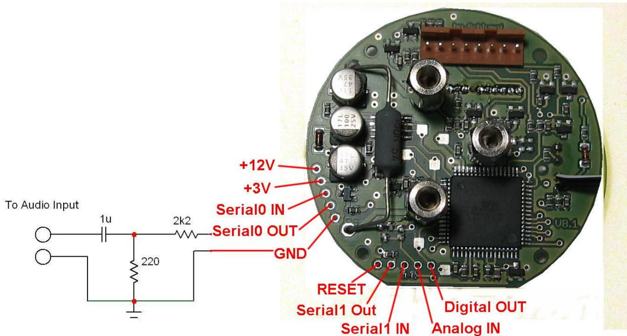
This function uses the same serial port as the GPS modification. It is not possible to run both at the same time.
