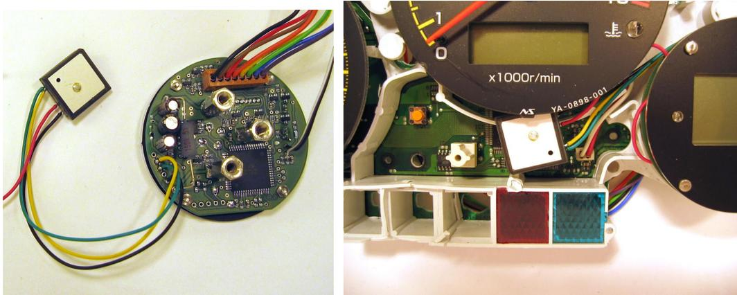
GPS support has to be enabled and set up in software in menu 2. Consult the user guide document for further details if needed. Enable, select baudrate and save. 4800 baud is a widely used standard. If set correctly message names will be shown in the upper right. Typically they are updated and altered every second:
