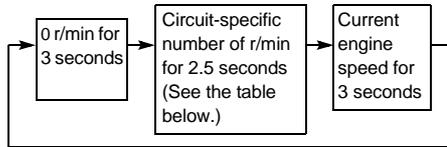
Use the chart below to identify the faulty electrical circuit.
